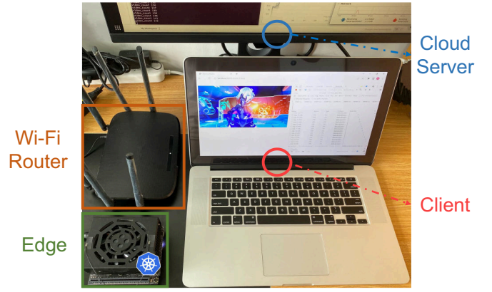
Fig. 7. Implementation of our serverless video streaming system prototype.
