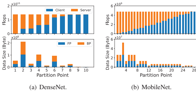
Fig. 4: The computing density and the amount of exchanged data of different training models (the number of trained data samples is 100).
